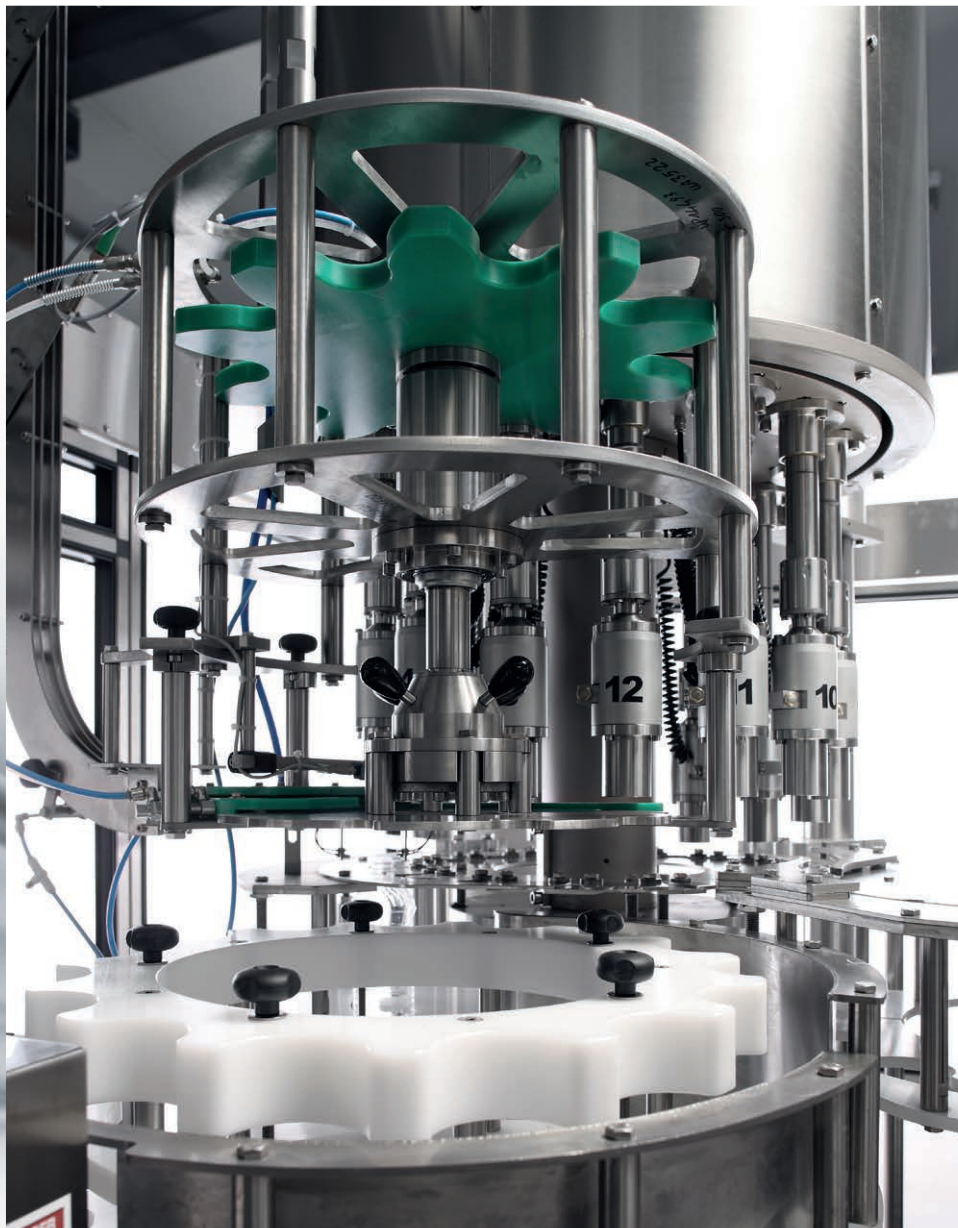
Cappers provided for each type of closure for edible oil industry (press-on, aluminium ROPP)
