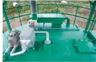
COMPO FUJI equipped the special heat exchanger which utilizes heat of fermentation in organic wastes. It makes water evaporate and warming air to send into the system. So, COMPO FUJI produce high efficiency fermentation without using heater.
